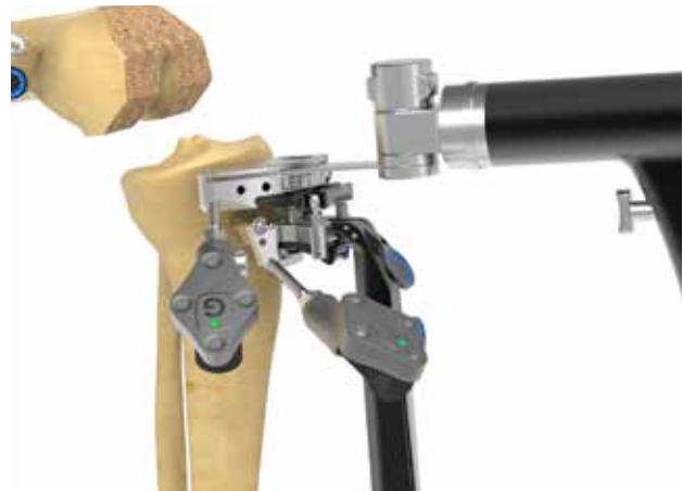
Figure 56 Invert Saw for Increased Access to Cutting Slot
