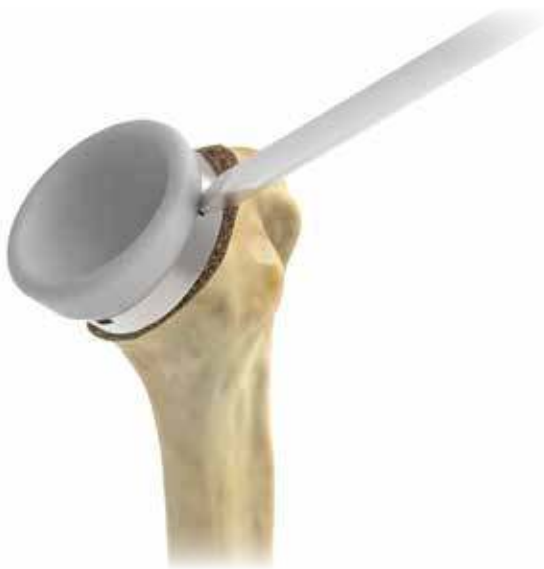
Figure 66 Humeral Liner Removal
