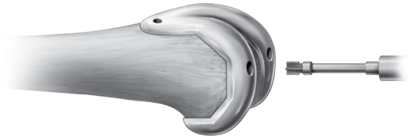
Figure 31 Prepare Femoral Peg Hole
