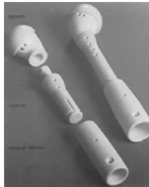
Figure 5 First reported modular humeral prosthesis (Salzer, 1979) 21
