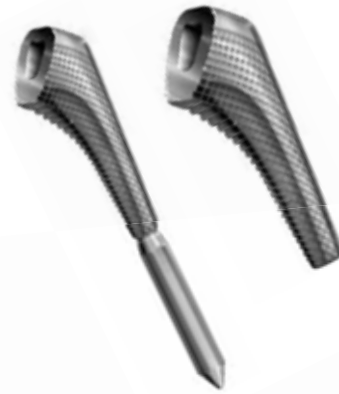
Figure 2 Extended Broach Tooth Geometry
