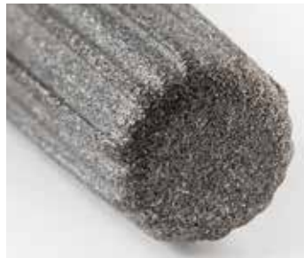
Figure 11 Grit Blast Surface Finish
