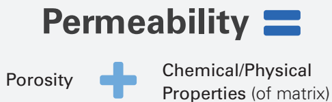
Figure 6. Permeability = Porosity + Chemical/Physical Properties (of matrix)
